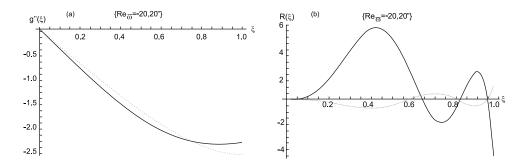
Figure 6: Plot of 3<sup>rd</sup> order OHAM solution (18) for  $g(\xi)$  and  $R(\xi)$  from wall injection to wall suction
