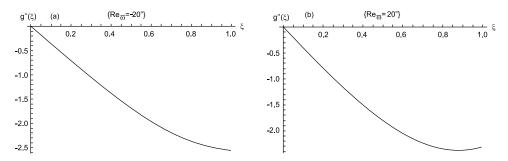
Figure 3:  $3^{rd}$  order OHAM solution (18) for  $g(\xi)$  with (a) wall injection, (b) wall suction
