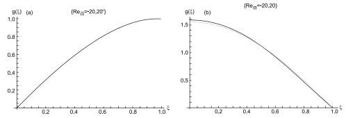
Figure 5: Plot of  $3^{rd}$  order OHAM solution (18) for  $g(\xi)$  and  $g(\xi)$  from wall injection to wall suction
